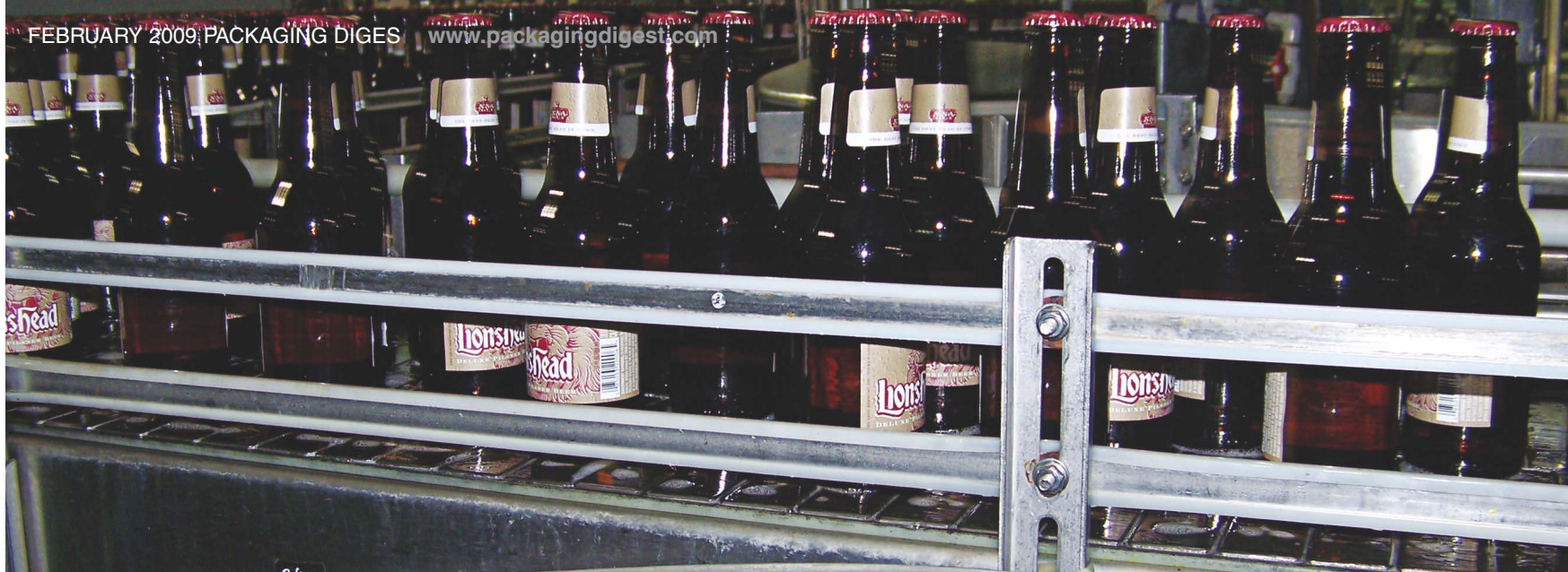
The brewery reconfigured its two bottling lines in 2001, and the new lines are capable of filling 400 bottles/min each.
